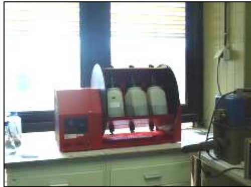
Figure 2 – Leaching test apparatus
