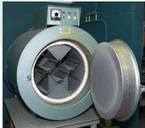
2 – Oven used to dry wet electrodes
