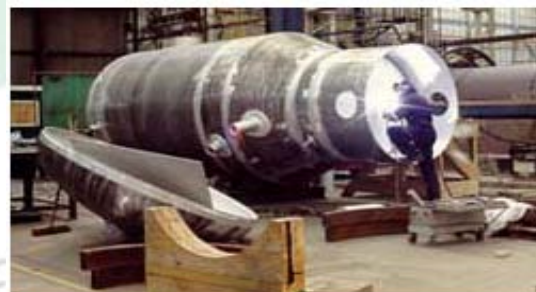
Fig.2 - AC TIG welding of aluminium cryogenic pressure vessel
