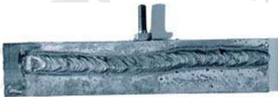
Fig. 1- Side deflection of arc.
