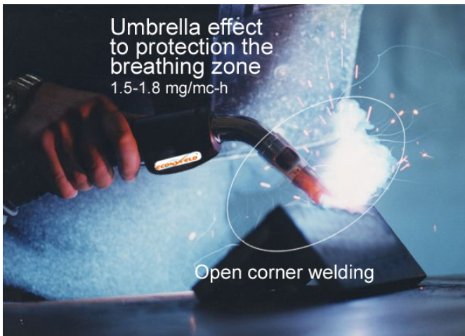
Figure 3: Example of application of the ECONWELD lightweight aspiration torch
